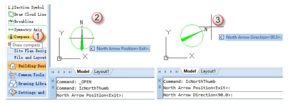
**Operation Guide for Drawing Compass**
