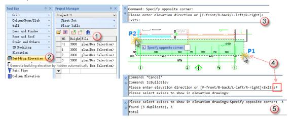
Operation Guide 1 for Elevation
