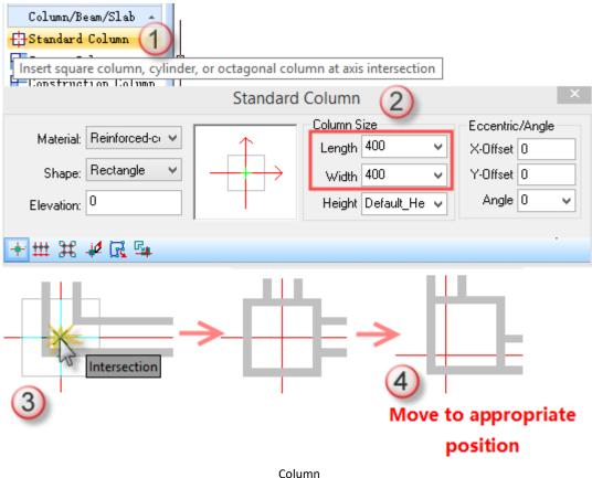
(2) The effect of the column is related to settings for materials, scale factors, and hatch mode. It is helpful to master settings for them when drawing or editing columns. View effect as below:
